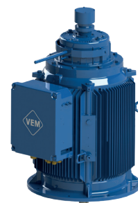
Three-phase asynchronous motor in non-ventilated version with electromagnetic spring-set brake and incremental encoder, type of protection IP 66
