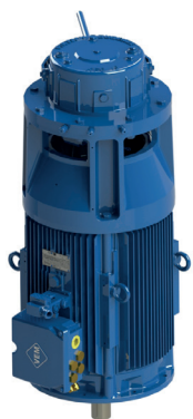
Three-phase asynchronous motor in non-ventilated version with electromagnetic spring-set brake and protected hollow shaft incremental encoder between motor housing and brake, type of protection IP 56
