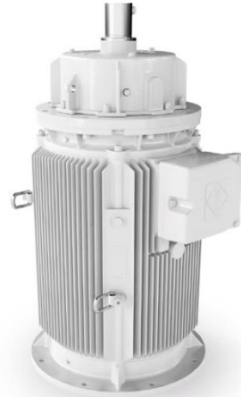
Three-phase asynchronous motor in non-ventilated version with electromagnetic spring-set brake and incremental encoder, type of protection IP 66
