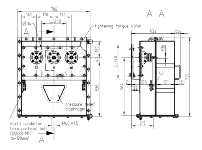
Explosion-proof three-phase asynchronous motors with squirrel-cage rotor for high voltage
