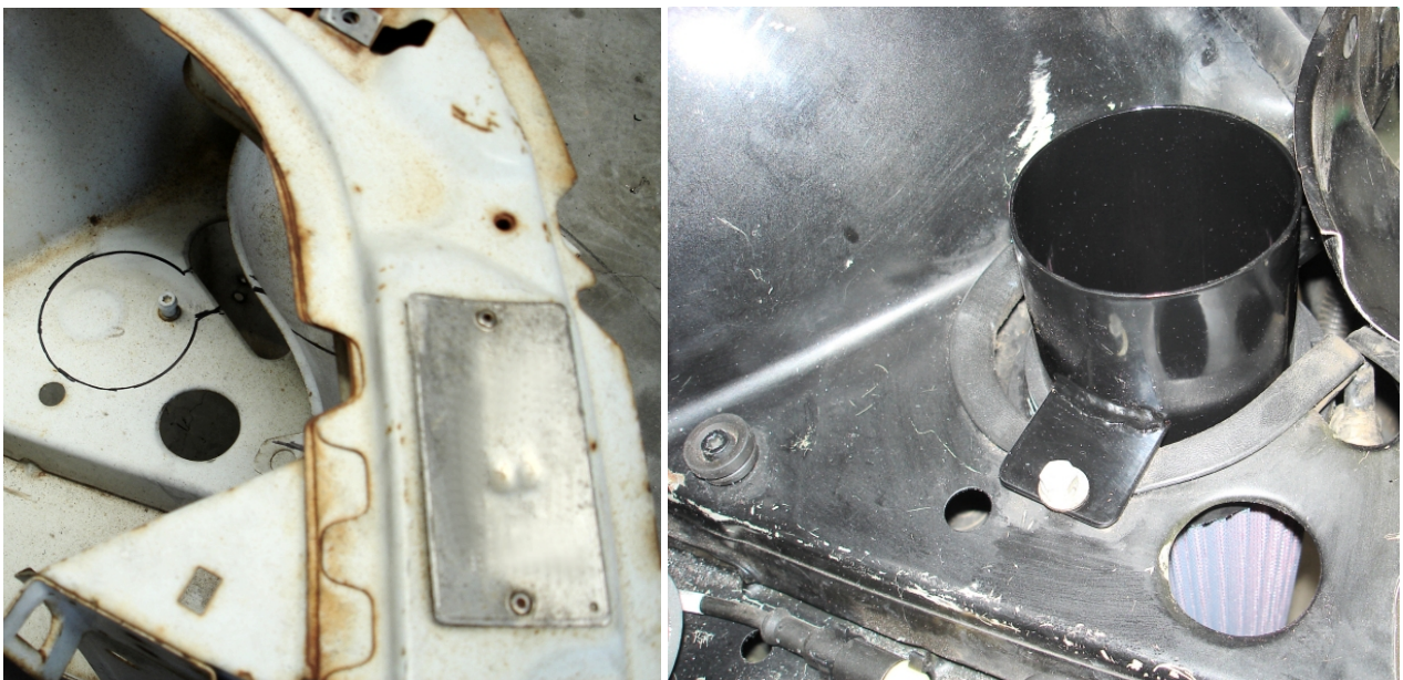
Image 9. Cut out hole for air filter
