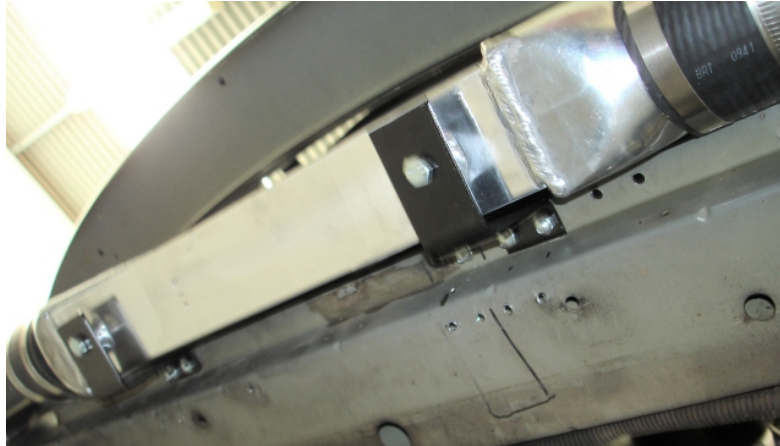
Image 4. Bottom Intercooler Brackets
