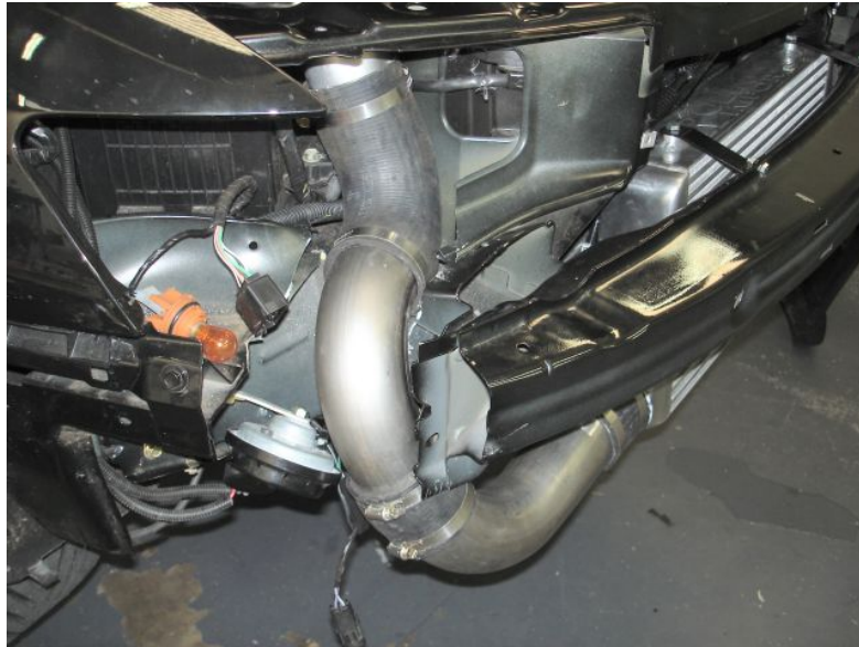
Image 6. Intercooler Pipework, Drivers Side Bottom
