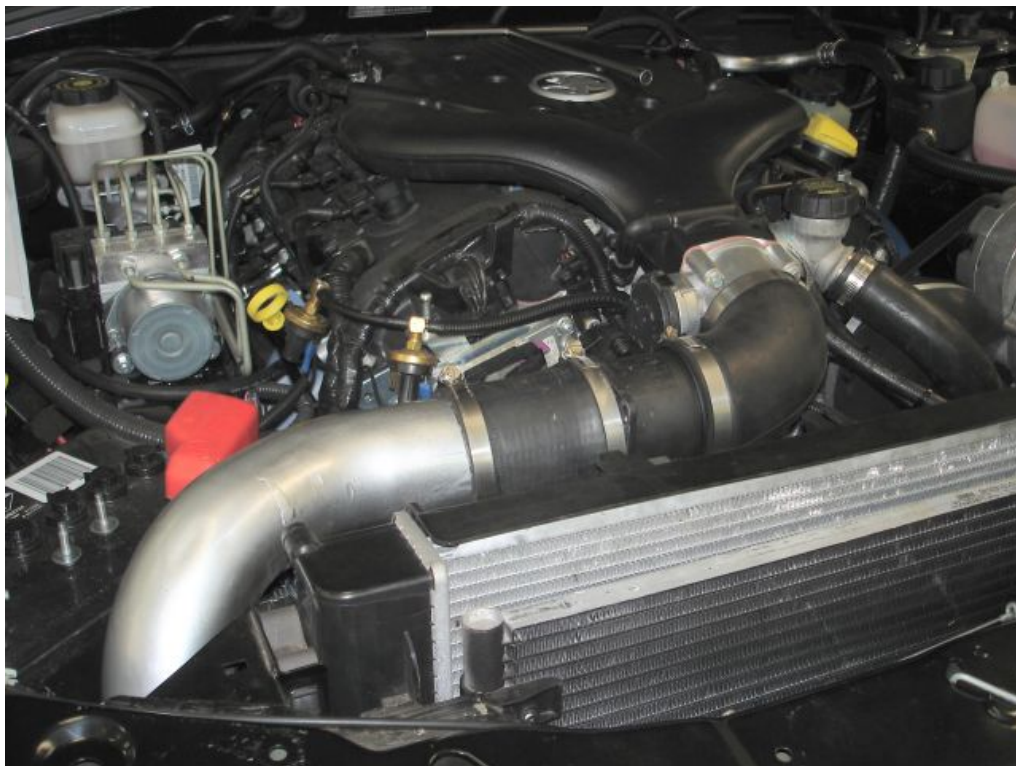
Image 7 – Intercooler Pipework, Drivers Side Top
