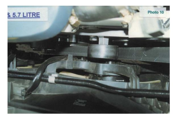
29. Re-fit radiator and fan assembly. Re-connect hoses and wiring. Fill radiator with coolant saved from drain. When motor is started, purge air filter system and complete top up of system. Check between cooling fans and engine that nothing is close, or that nothing will rub if motor comes forward a small amount.
