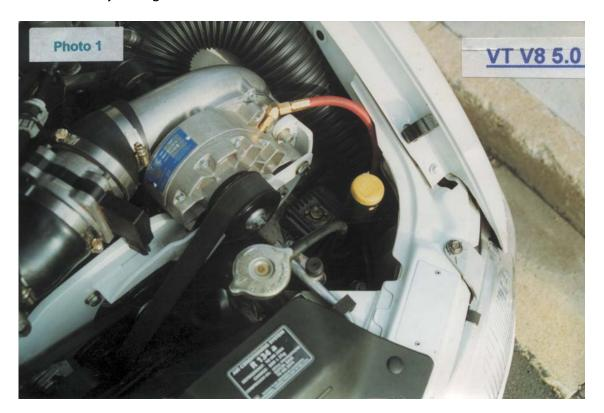
5. Wither supercharger and alternator idler bolt and pulley fitted to bracket, fit bracket to motor using new bracket bolts supplied, with spring and flat washers:
