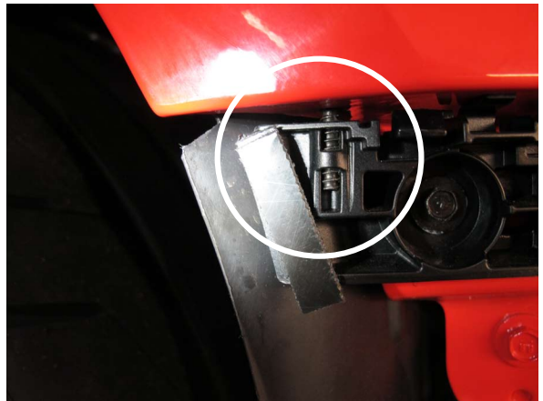
Fig. 1-h: Bumper Corner Fastener (Bumper Removed)
