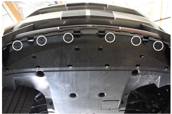
Fig. 1-g: Remove Front Belly Pan Screws
