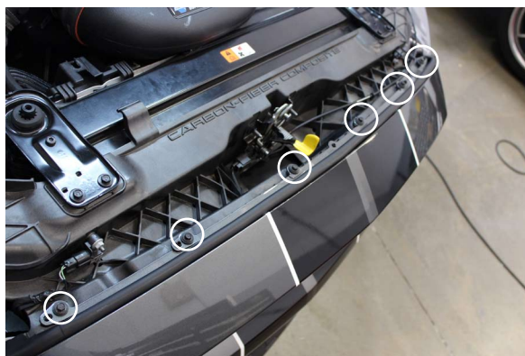
Fig. 1-a: Remove Bumper Cover Fasteners
