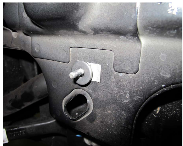
Fig. 10-i: Install 5/16 Washer To Mounting Stud
