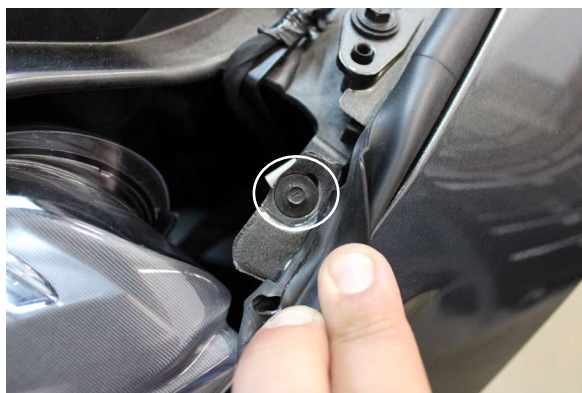
Fig. 1-b: Remove 5.5mm-Headed Fastener
