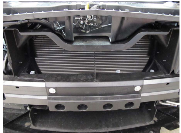
Fig. 1-j: Remove Radiator Shroud
