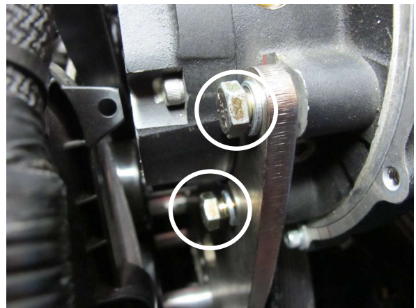
Fig. 3-q: Mount Supercharger To Bracket & Secure
