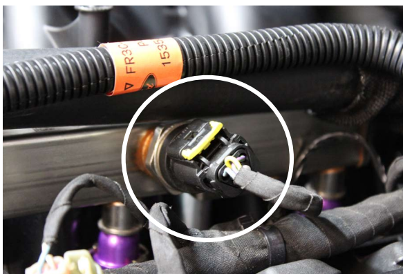
Fig. 6-c: Remove Fuel injector Rail Assembly
