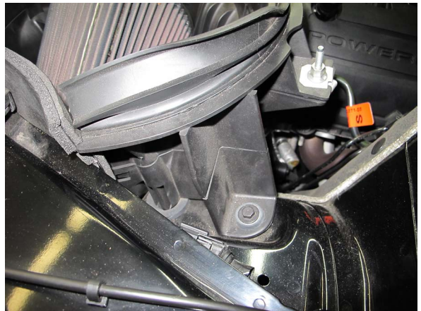
Fig. 1-n: Unplug MAF & Remove Air Inlet Assembly
