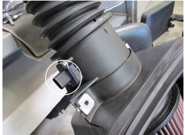
Fig. 1-s: MAF Insert (shown with OEM airbox removed)
