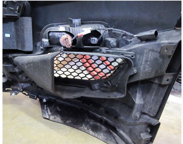
Fig. 10-m: Remove Transmission Cooler Duct
