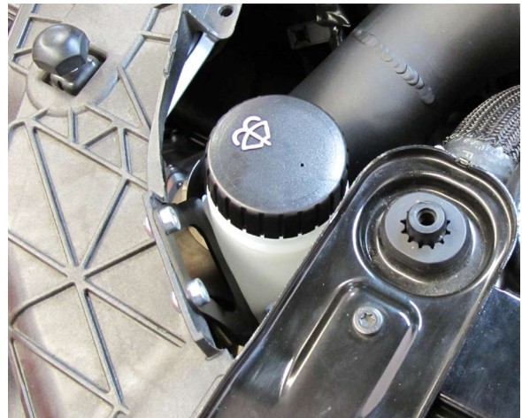
Fig. 10-g: Mount Remote Fill Bracket
