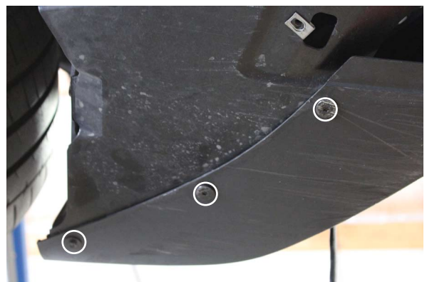
Fig. 1-f: Remove Screws Securing Front Bumper Corners
