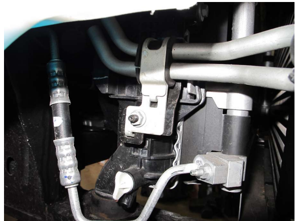
Fig. 10-b: Remove Transmission Cooler Lines From Mount
