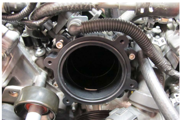
Fig. 3-u: Clean T-Body Flange & Verify O-Ring Placement
