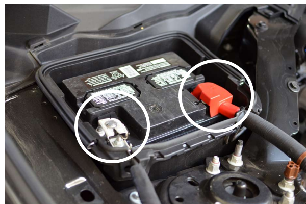
Fig. 2-e: Unplug Battery Leads
