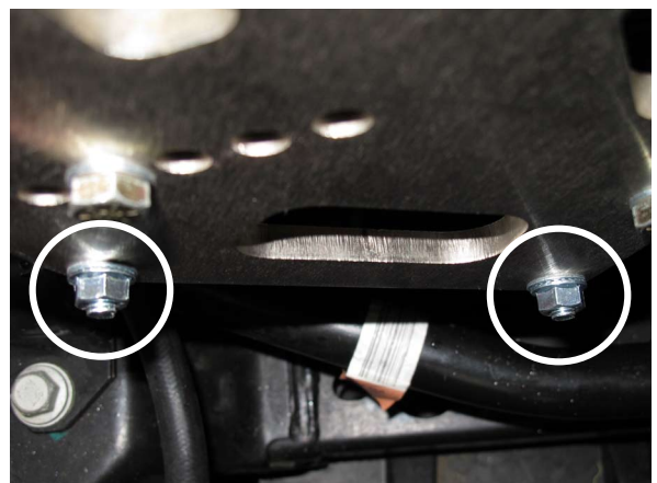
Fig. 3-l: Secure Lower Mounting Bracket Fasteners
