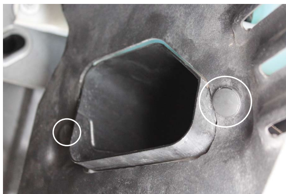
Fig. 1-c: Remove Fender Liner Fasteners
