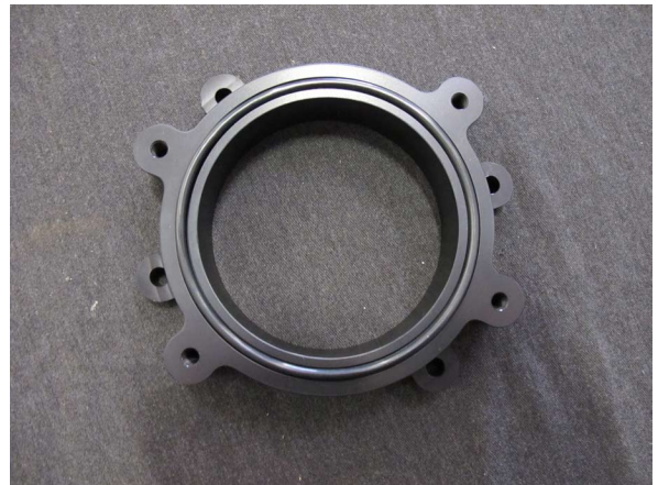
Fig. 3-t: Place O-Ring In Anodized Spacer
