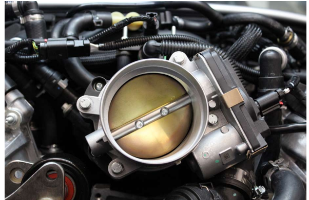
Fig. 3-v: Re-Install T-Body 180° From Original Orientation
