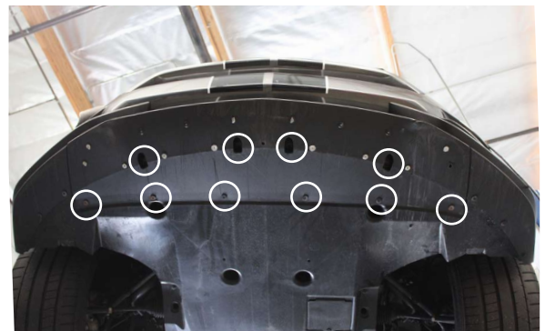
Fig. 1-e: Remove Front Splitter
