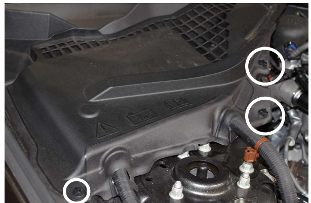
Fig. 2-c: Remove Battery Cover
