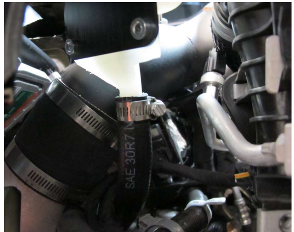
Fig. 10-k: Secure 5/8 Hose To Remote Fill Reservoir
