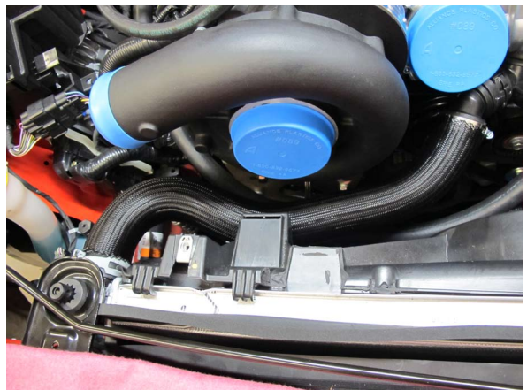
Fig. 7-c: Upper Radiator Hose (New Configuration)
