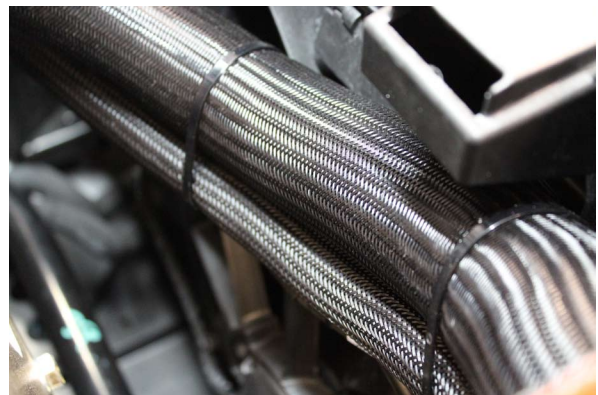
Fig. 7-o: 3/4" Coolant Hose Routing
