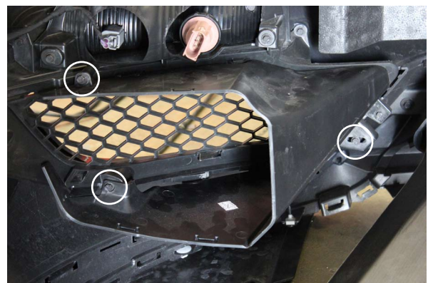
Fig. 5-o: Remove Oil Cooler Duct
