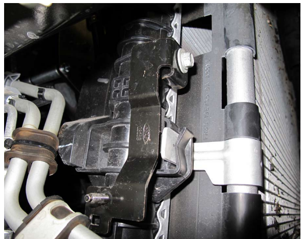
Fig. 10-c: Remove Transmission Cooler Lines Mount From Radiator
