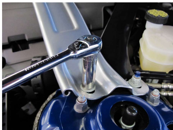
Fig. 2-d: Remove Strut Tower Brace
