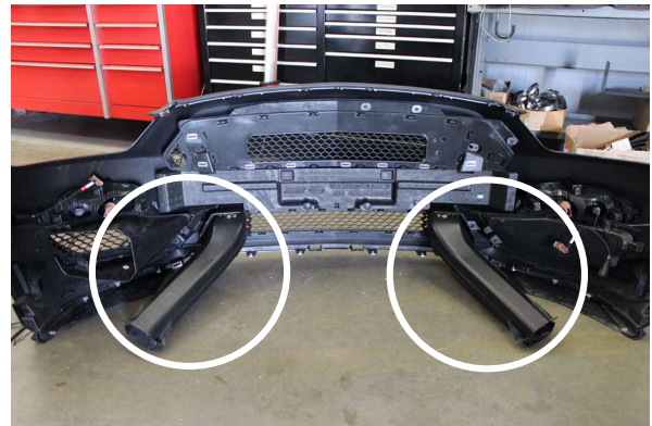
Fig. 5-n: Remove Brake Cooling Ducts
