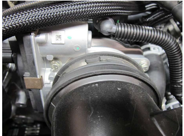
Fig. 1-m: Loosen Hose Clamp & Detach Breather Hoses
