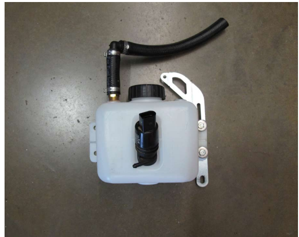
Fig. 10-h: Assemble Windshield Washer Reservoir As Shown
