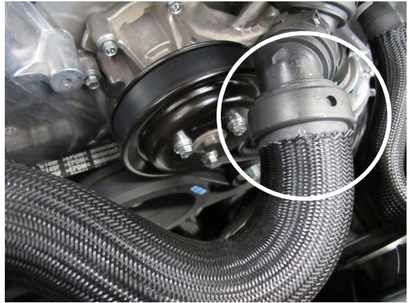
Fig. 7-b: Cut Plastic Hose Clamp
