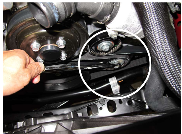
Fig. 1-r: Remove Accessory Drive Belt
