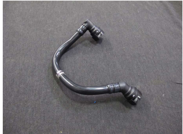
Fig. 4-a: OEM Passenger Side PCV Hose (Fittings Removed)
