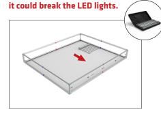
**Step 14: Turn. Position. Lock.** Insert tensioning pole into the bottom of display. Keep the pole flat until the entire pole fits inside the frame. **Turn** the pole 45°. **Position** and
