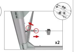
**Step 5:** Move to the center of cable and hand tighten remaining turn buckle to remove any remaining slack. Do not over tighten.
