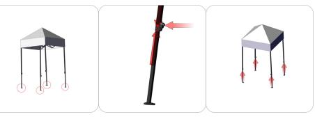
The frame will have four slide locks, one for each corner. When the tent scissor frame is fully extended; make sure the prong of the slide lock snaps into the tube locator hole. Press the lever on the slide lock to disengage the prong from the tube allowing to slide the lock up or down during assembly.
