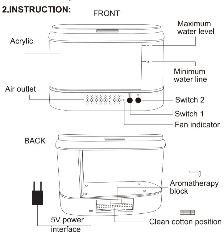
1. Connect USB adapter into the DC 5V power interface, the water pump start work for water recycle and enhance oxygenation.
