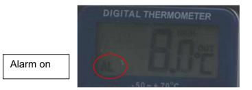
**NOTE:** While setting limits, if the current temp is outside the set limit, the alarm will sound. Press any button to stop the alarm sounding.
