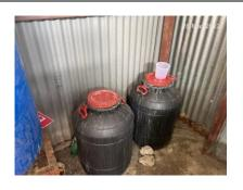
Proper labelling, secondary containment and eye wash station was not provided to chemical drums
