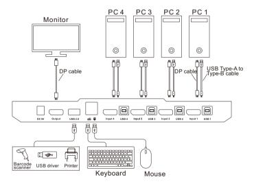
**Note:** The keyboard hot key is available only when the keyboard is connected to this dedicated port.
