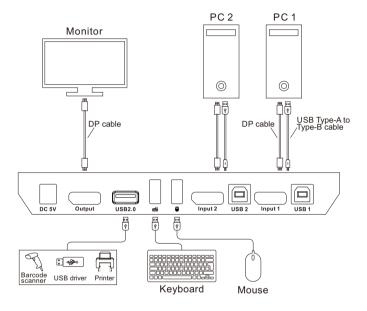
**Note:** The keyboard hot key is available only when the keyboard is connected to this dedicated port.
