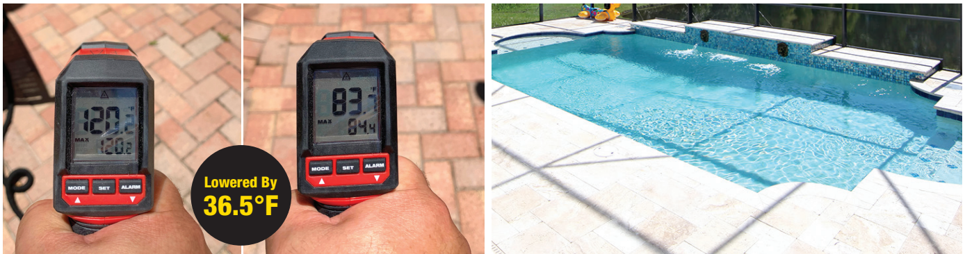
Before coating air temp 83°F. surface temp 120.2°F After coating air temp 85°F. surface temp 83.7°F
