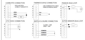
3-wire RTD Temperature sensors are normally wired with 2 red and 1 white conductor. Connect the white conductor to RTD1, then 1 red to RTD2 and 1 red to RTD3. Do not connector RTD2 and RTD3 together at the connector.
