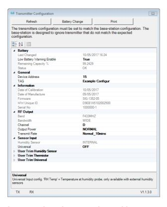
Note: Each transmitter must have its own unique address or conflicts will arise giving false readings. Transmitters must be enabled in the Basestation using the spYconfig software. Signals arriving at the Basestation which have not been enabled within the Base-station configuration will be ignored.
