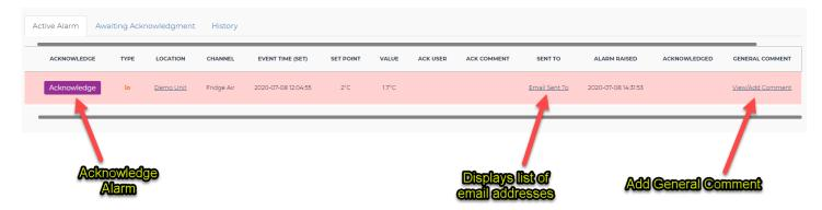
When acknowledging an alarm, a popup window will appear to give a comment. The alarm background colour will then turn yellow. It will also be pushed down the list, below any non-acknowledged alarms. Additional information will show who acknowledged the alarm and when the alarm was acknowledged.
