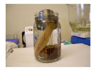
Apply the maximum vacuum to the chamber that your system will permit. The length of time required at vacuum will vary depending on the system and the type/size of wood and will require some experimentation. A high vacuum (<10 mBar) high flow system (>27 cfm) running continuously can fully evacuate spalted pen blanks in about 20 minutes or until air bubbles rising stops; other systems may require hours or even days at vacuum.
