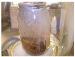
Once the vacuum stage is completed, release the vacuum to permit the wood to absorb the stabilizer. With the lid removed, you should check to ensure the level of the stabilizer is still above the wood. If not, add more stabilizer and repeat the vacuum process. The wood should be permitted to soak in the stabilizer for at least 20 minutes. More time may be required for dense woods.
