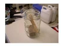
Place your wood pieces in a container and weight them down to prevent floating. The container should be tall enough to prevent foaming over the sides during stabilization.
