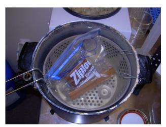
Upon completion of curing, permit the wood to air-cool to room temperature. Trying to cool the wood rapidly will adversely affect the hardness of the cured stabilizer.
