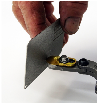
Sharpening the Pro-Forme Powerhead with an Eze Lap diamond lap stone
