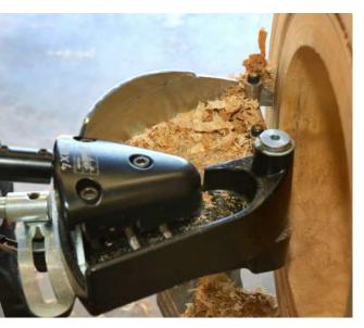
When coring hard and dense wood there is a risk of and the lathe bindina This be stalling. can prevented by cutting a wide channel on the inside of the bowl to create more clearance for the cutter. Create the wider channel by backing out of a cut to clear chips, then pull slightly on the cutter when going back to the cut and then retract and push on the cutter bar getting back to the cut. This provides an extra 1/64" clearance on each side.
