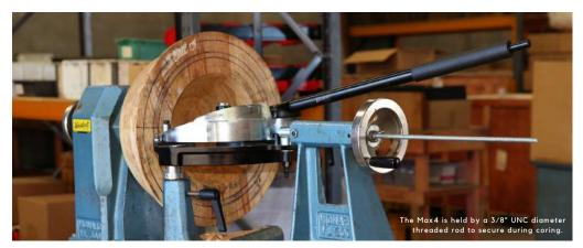
The Bowlsaver Max4 is designed to cut in an exact semi-circle which has a radius that you can measure from the central rotation post of the Max4.
