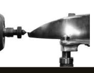
3. Position the Tool Post so the Blade cutter is centered with the point of the drive spur, or slightly above as illustrated (this assumes that when the Blade is extended in the End Grain of the wood that the Blade is now at center). Tighten the Tool Rest locking handle. Slide the shaft collar down the support post and then tighten the grub screw.
