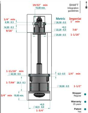
All measurements in mm. Tolerances shown are for mounting into wooden products. Minimum 6mm wall thickness around ribs recommended for wooden products.
