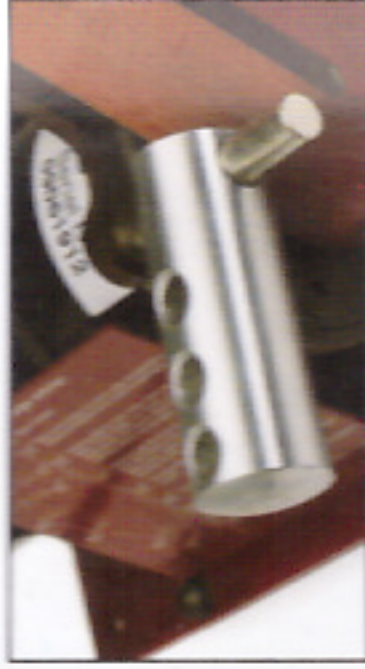
Long grind jig holes 3, 2 & 1
