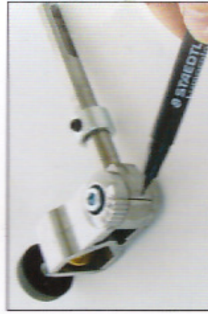
Finger nail profile arm with adjustable collar (AC)
