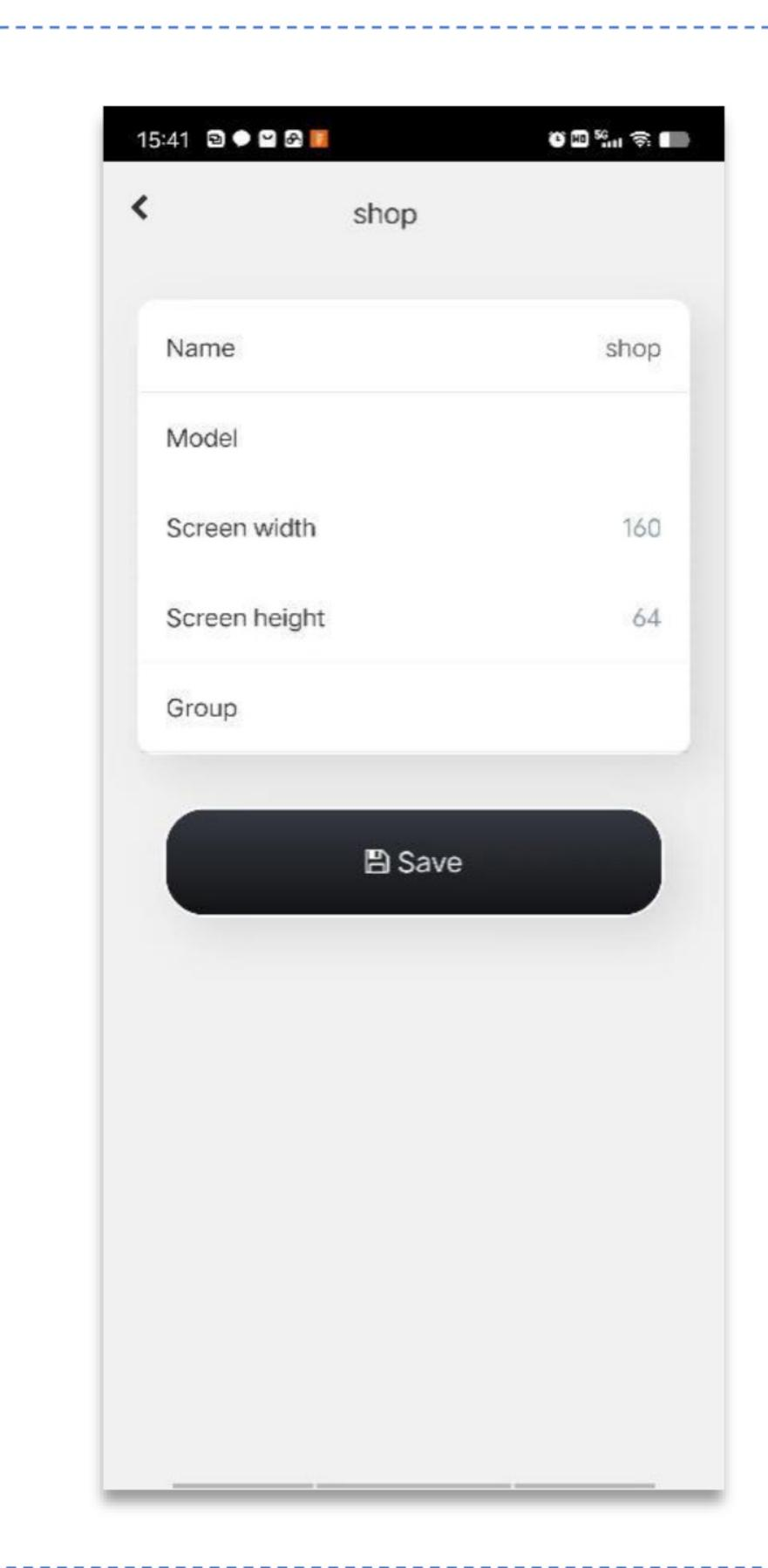
Under the Device Information interface, you can modify the device name and device group.
