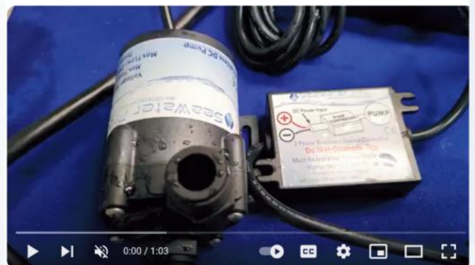
SeaWater Pro - watermaker brushless boost pump protection logic.
