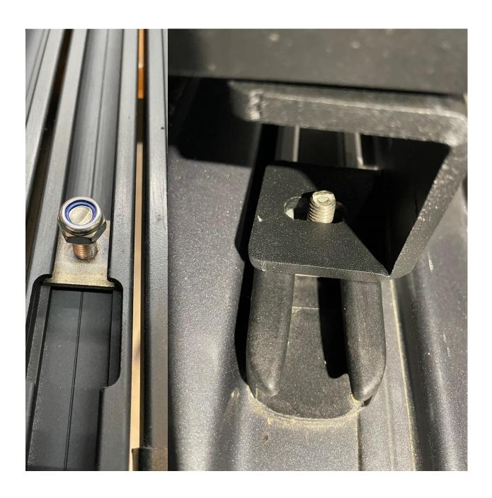
Then finish the rack installation by tightening the self locking nuts for the track bolts.
