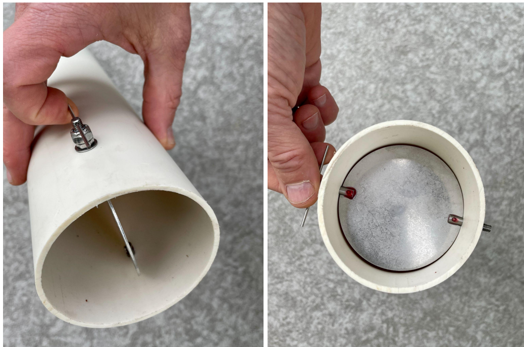
Comfort damper valve open on left and closed on right
