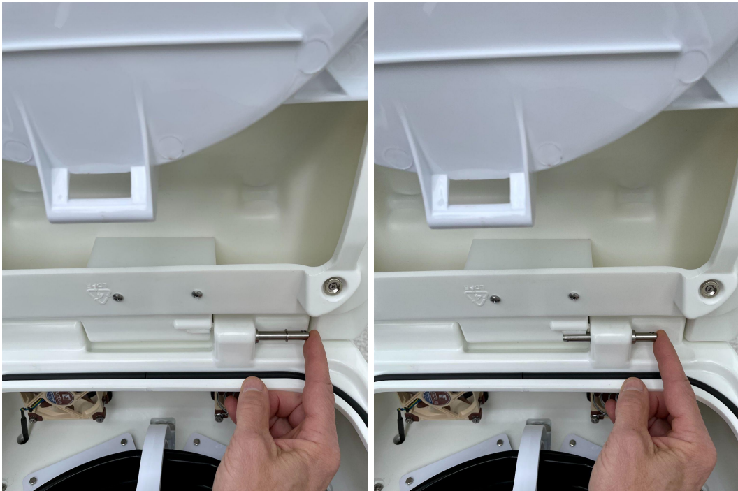
Hold the seat open with the latch pin as shown
