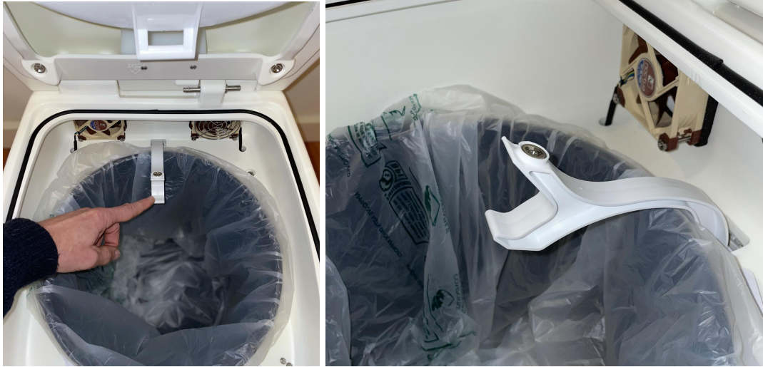
Here the trap door arm is shown over the waste container
