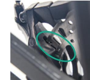
5.3 Screw the left and right nut together with two wrenches and make sure the front wheel is fixed to the front fork tightly.
