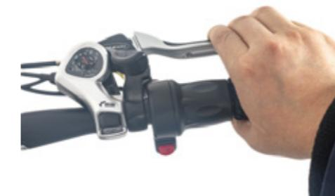
(8) Press the red button and turn the throttle to drive the bike.
