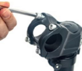
4.2 Install the handlebar to the handle stem and screw the four bolts again with matching wrench. During the installation, adjust the handlebar to an appropriate angle so that the bike can be operated comfortably.
