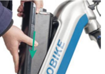
10.2 Press the battery a little hard until the battery is pushed into the battery compartment.
