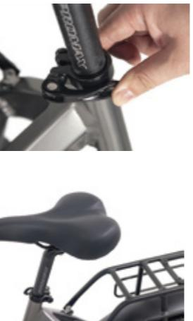
15.1 Move the saddle up or down to your desired height,screw the handle to make it tight or loose, then fold the saddle quick release to make the saddle post fixed tightly.
