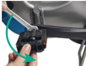
8.3 Screw the right pedal<sup>①</sup> bolt into the right crank<sup>②</sup> with a wrench clockwise.
