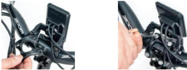
4.3 Make sure the four bolts are screwed tightly and the handlebar cannot be moved.
