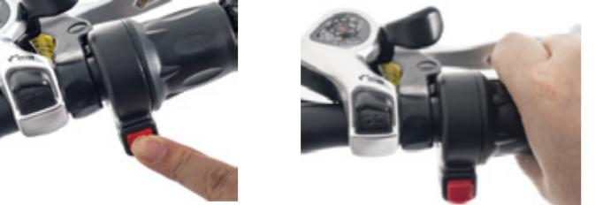
(9) Switch the shifter by "+" and "-"button to adjust the speed for fitting with different road conditions.
