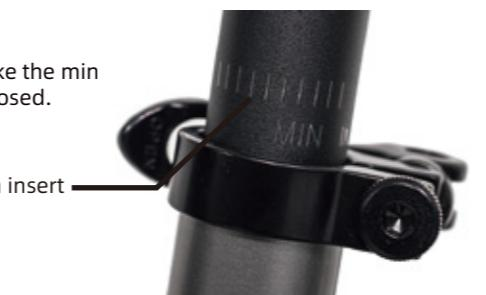
15.2 Do not make the min insert mark exposed.
