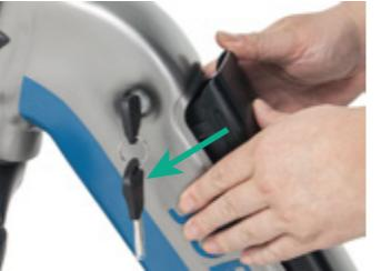
10.3 Turn the key clockwise to the end and then the battery is locked.
