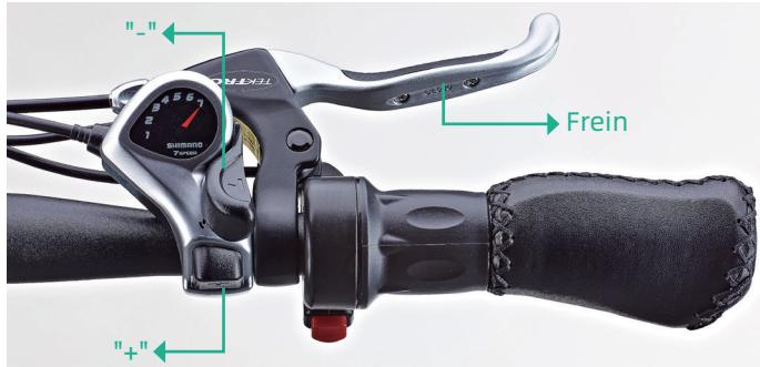
If the bike you received is without the switch, just twist the throttle to start directly.
