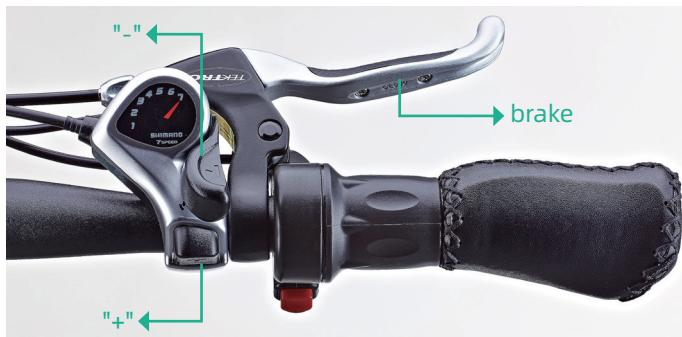
If the bike you received is without the switch, just twist the throttle to start directly.
