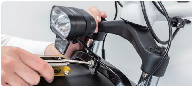
5.2 Adjust the headlight to a proper angle by this way: loosen the adjusting bolt with a cross-head screwdriver, adjust the headlight tilt angle to the best position, and then tighten the bolt.
