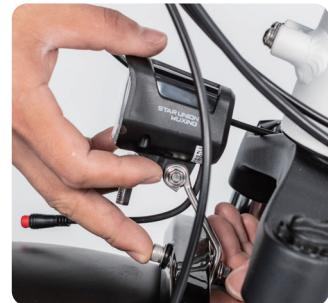
5.2 Adjust the headlight to a proper angle by this way: loosen the adjusting bolt with a cross-head screwdriver, adjust the headlight tilt angle to the best position, and then tighten the bolt.
