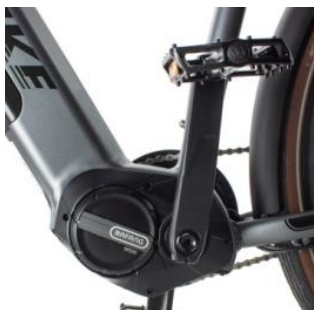
Left pedal tightens counter clockwise
