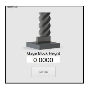
Tool 4 is ready to have a length offset applied. It will be the value that is shown in the Z DRO. To set this offset for Tool 4, the "Set Tool" button will be used. This is located to the right of the "Z Offset" set button in the Offsets tab.
