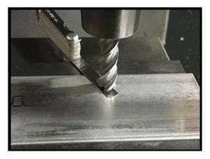
Tool 4 has been called and its offsets are active. Using the same method as the previous tool, manually jog Tool 4 in position on the work surface using a shim.
