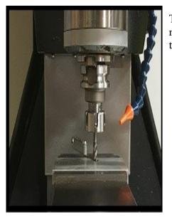
Tool 3 has been called and its offsets are active. Using the same method as the previous tool, manually jog Tool 3 in position on the work surface using a shim.
