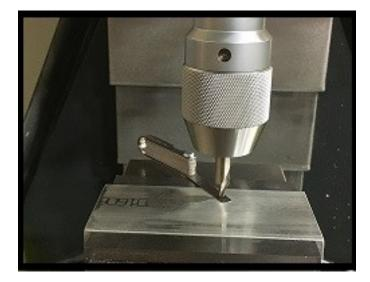
Tool 1 was loaded in to the tool holder and has been manually jogged down to the top of the piece of material that is slated to be machined. In the picture, a shim is used to finish bringing the tool down onto the work piece. This is used as an indicator to know when the tool begins to touch, and to avoid damaging the tool on the work piece.
