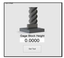
Tool 3 is ready to have a length offset applied. It will be the value that is shown in the Z DRO. To set this offset for Tool 3, the "Set Tool" button will be used. This is located to the right of the "Z Offset" set button in the Offsets tab.
