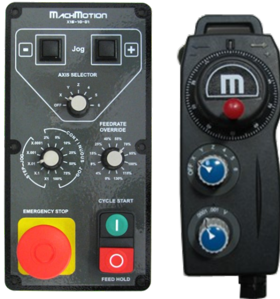
Figure 3-6: Control panel and pendant examples
