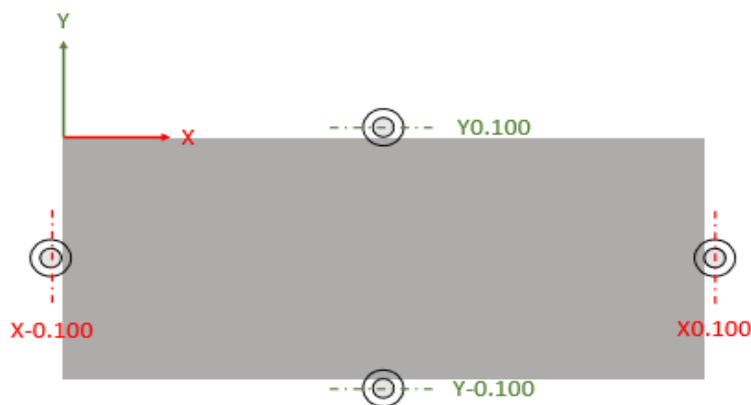
Figure 3-14: Touch off location for 0.200 inch diameter edge finder
