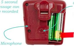
*Use a pointed* object to press down recording button
