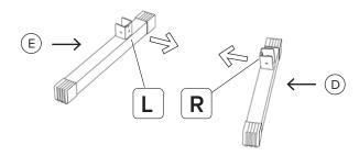
Place the left (E) and right (D) base parts on the floor, making sure that "L" and "R" marks are facing each other.
