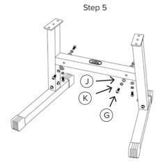
Use one of the hex keys to fasten the centerbeam with 6 bolts (G), 6 spring washers (K) and 6 flat washers (J). Make sure the the spring washer is closest to the bolt head.
