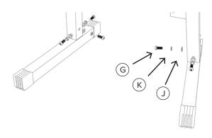
Use one of the hex keys (L) to fasten the pillars with 6 bolts (G), 6 spring washers (K) and 6 flat washers (J). Make sure that the spring washer is closest to the bolt head.
