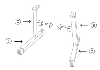
Mount the left pillar (C) on the left base and the right pillar (B) on the right base, making sure that the connectors on the pillars are facing each other.
