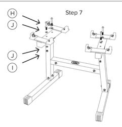
Use one of the hex keys (L) and the universal tool (M) to fasten the trays with 4 bolts (H), 4 flat washers (J) and 4 bolts (I).
