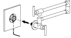
Wrap the PTFE tape onto the adapter, screw the Tap body to the proper position, then lock the hex socket screws with a Hex key.
