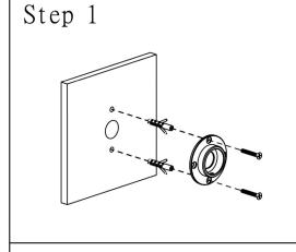
Choose the appropriate drilling location to fix the Base on the wall with a drill and a screwdriver.
