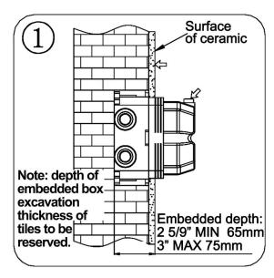
3. As shown in the figure, the inlet and outlet pipes should be embedded well, pay attention to the up and down, left and right directions on the embedded box.
