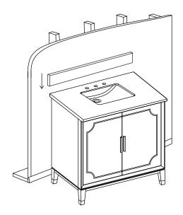
Finally,place the bottom side of back splash with sealant onto the counter top and check alignment of back splash.
