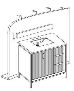
Finally,place the bottom side of back splash with sealant onto the counter top and check alignment of back splash.
