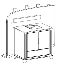
Finally,place the bottom side of back splash with sealant onto the counter top and check alignment of back splash.
