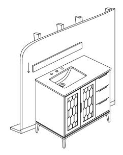
Finally, place the bottom side of back splash with sealant onto the counter top and check alignment of back splash.
