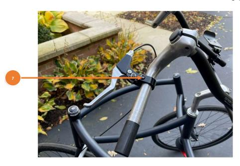
• While holding the hand grips, with your forearms flat in the forearm supports, place the brake lever at the angle that allows you to operate the brakes most easily and comfortably.
