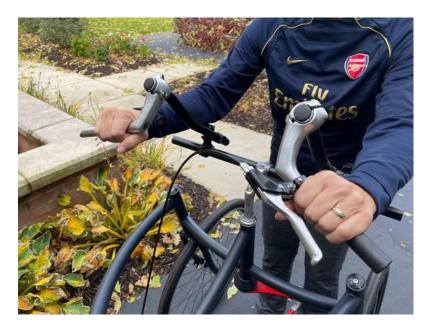
• Tighten the screw to hold the brake firmly in its intended position (ref. 7, above).
