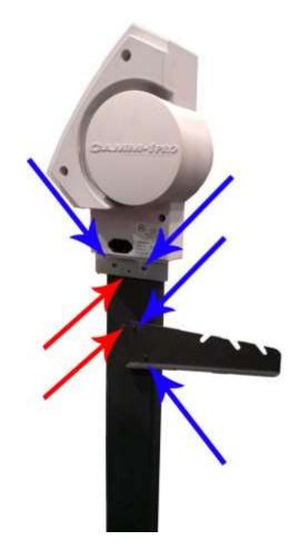
The red arrows indicate the locations of the 4 (2 per Fusion Wheel and Bracket Assembly) M4x20 screws with washers to be installed with the Fusion Wheel and Bracket Assembly. Example shown below.
