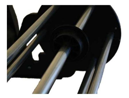
8. Slide the desired film or vinyl onto the Chrome Tube with a Cone on each end and tighten the set screw with the 1/8" Coated Hex Key. Once you have determined your desired location for the Cones so that your material is lined up with your plotters' feed rollers, you will seldom need to adjust the position of the Cones on the right side of the Chrome Tube. At this time, simply remove the left Cone and exchange your media (film or vinyl). Reinstall the left Cone and no realignment is necessary.
