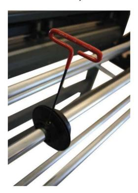
9. Insert the end of the tube that does not have the metal stop rings on it into one of the Left Side wheel holes. Pull back the right side retaining spring lever and lock the Chrome Tube into the Right Side Wheel with the metal stops fitting around each side of the wheel. Release the lever.
