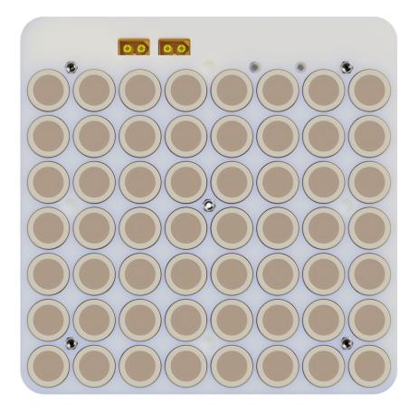
Cells should be inserted into the box with the positive side down and the negative side up, as shown in the picture above. Alternatively, you can remember that the PCB springs should always touch the flat side of the cell.
