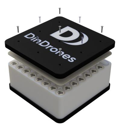
DinBox is a field charging solution designed for RC enthusiasts who require independence, efficiency, and mobility. It contains 56 x 5000mAh 21700 cells, forming a 4s14p battery capable of charging 32 x 1400mAh 6s or 34 x 1300mAh 6s batteries from 0 to 100%. In real-life terms, this means it can charge approximately 40-50 batteries, as fully discharging batteries to 0% is detrimental.
