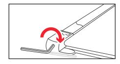
Note: Please remove the safety key and unplug the power cord. The running belt will loosen over time. A loose running belt will not function properly. Use the L-Wrench turn both rear idler bolts clockwise 1/4 of a turn to tighten the running belt. Then plug in the power cord, connect the safety key, run the treadmill for 3 minutes. Repeat until the running belt is centered.
