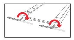
Note: A running belt that is too tight can cause damage to the belt itself and its rollers. Strange noises are an indication your belt is too tight and must be loosened for a safe experience. Note: Search "REDLIRO" on YouTube to find videos on how to adjust the running belt.
