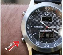
Timer: Set minutes on Select/Reset button and start and stop on right side button Start/Stop.
