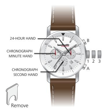
Remove the **plastic stopper** underneath the crown. Then push the crown back in to activate the battery.
