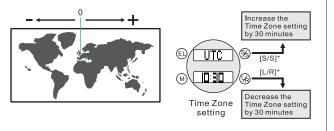
Note: Hold down the [S/S] or [L/R] button to change value at higher speed
