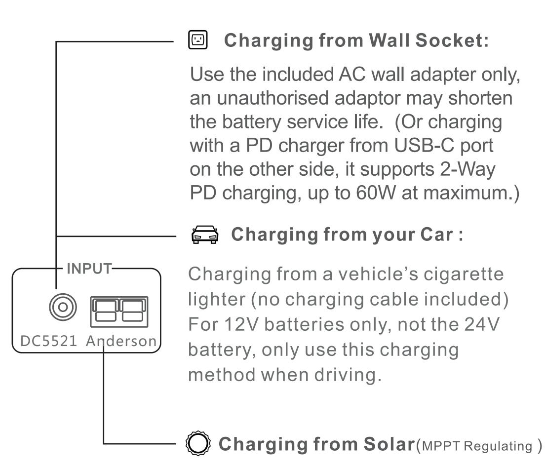
Charging from CAMPRITE Australia's fold-able solar panel/solar modules 60-100W, use MC4/DC5525 to Anderson cable. Different solar panels require different charging adapter to build connection, solar charging cable is not included. If in doubt, please email us for assistance
