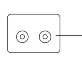
2 x DC: for LED lamps, or any other devices required no more than 12V working voltage. (DC 5.5x2.5 mm socket, single port supply no more than 12V5A.)
