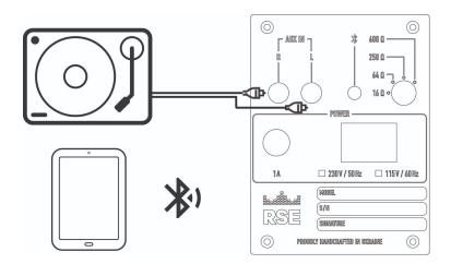
The RSE HA13S is equipped with unbalanced RCA connectors for input and TRS (Jack) 6.3mm output connections.
