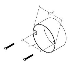
The backplates on this fixture are 4 inches in diameter and are made of solid metal (not pressed) so junction boxes must be flush with wall surface.
